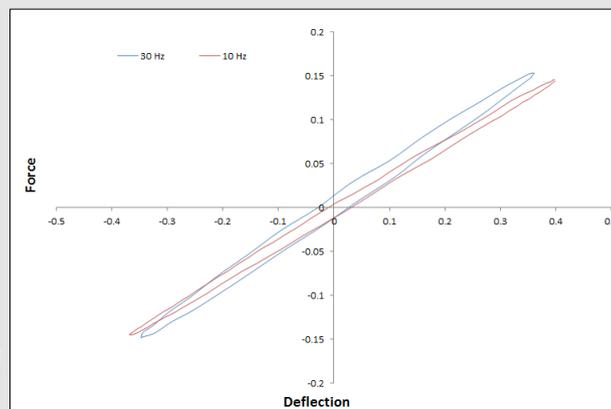
Figure 1: Load vs deflection curve of a rubber isolator under oscillating compression at 10 Hz & 30 Hz
