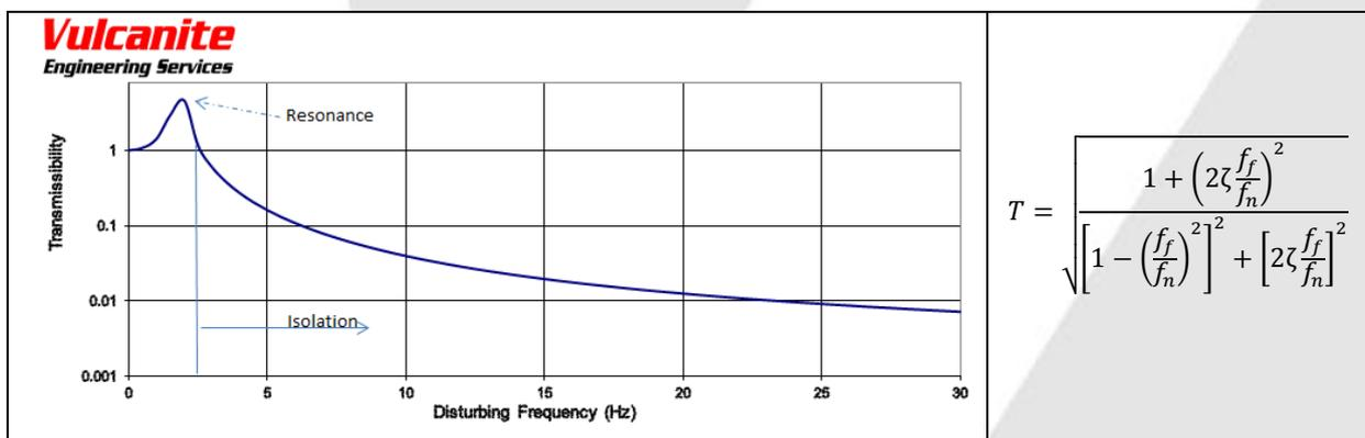
Figure 2: Typical Transmissibility curve of a rubber isolator
